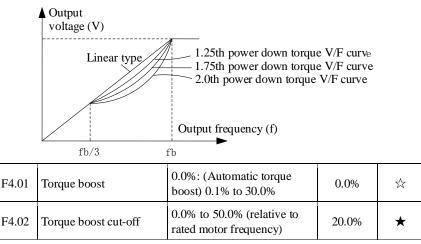
Torque boost is mainly used in below cutoff frequency (F4.02), V/F curve after boosting is as shown below, the torque boost can improve the characteristics of V/F frequency torque.
