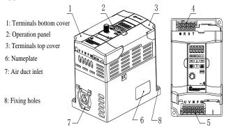
4: Inverter power input terminals5: Inverter output terminals
